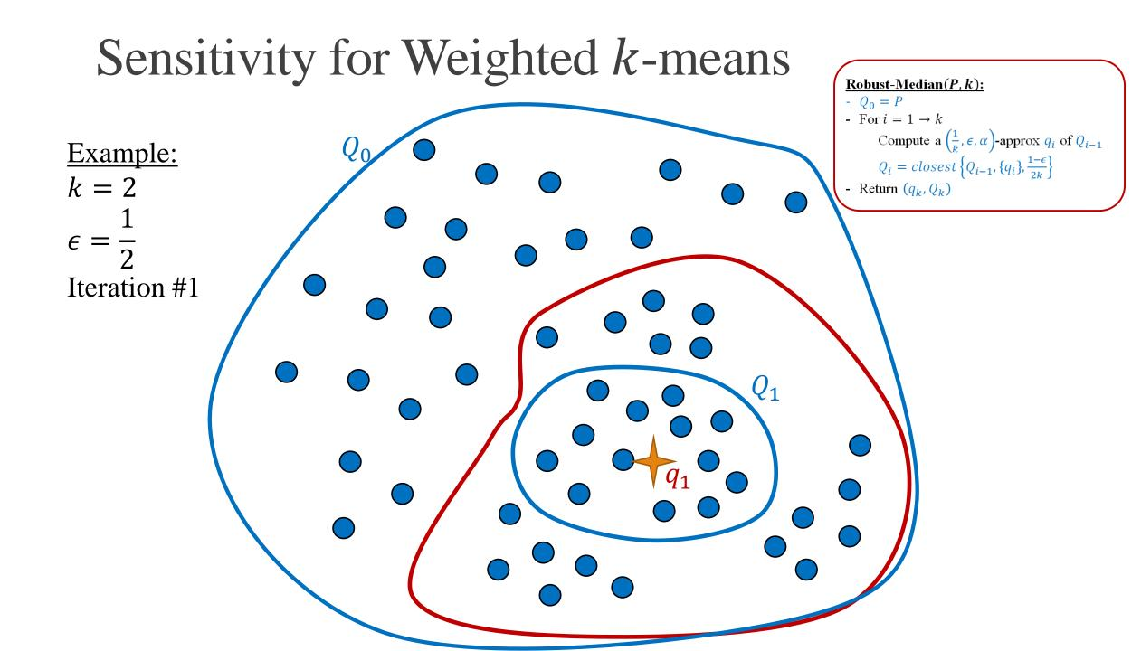
$$\begin{array}{l} \displaystyle \frac{\text{Robust-Median}(P,k):}{P} \\ \hline Q_0 = P \\ \hline \text{For } i = 1 \rightarrow k \\ & \text{Compute a } \left(\frac{1}{k}, \epsilon, \alpha\right) \text{-approx } q_i \text{ of } Q_{i-1} \\ & Q_i = closest \left\{Q_{i-1}, \{q_i\}, \frac{1-\epsilon}{2k}\right\} \\ \hline \text{Return } (q_k, Q_k) \end{array}$$
