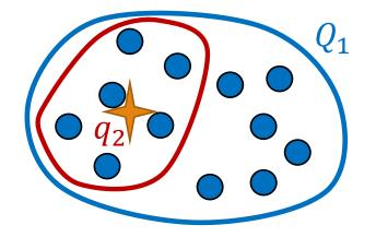
$$\begin{array}{l} \displaystyle \frac{\text{Robust-Median}(P,k):}{P} \\ \hline Q_0 = P \\ \hline \text{For } i = 1 \rightarrow k \\ & \text{Compute a } \left(\frac{1}{k}, \epsilon, \alpha\right) \text{-approx } q_i \text{ of } Q_{i-1} \\ & Q_i = closest \left\{Q_{i-1}, \{q_i\}, \frac{1-\epsilon}{2k}\right\} \\ \hline \text{Return } (q_k, Q_k) \end{array}$$
